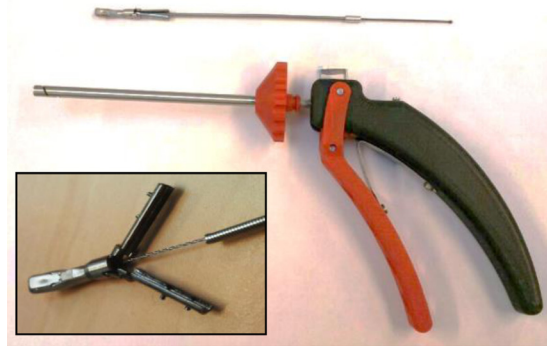
Fig. 4 Steerable punch dismantled into tip assembly, outer tube with wheel and handle. Opening of the hinge results in better access to all openings for cleaning and inspection.
